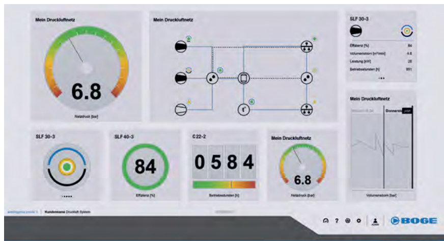
The comprehensive visualisation of the airtelligence provis 3 clearly displays status values and consumption processes of the compressors, which can be retrieved from anywhere. Image: BOGE KOMPRESSOREN.
